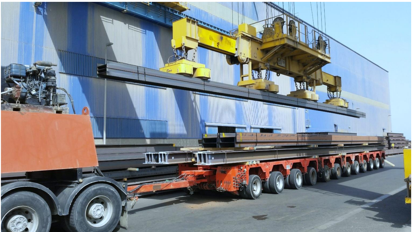
Fig: Structural Steel Sections Loading Activity
