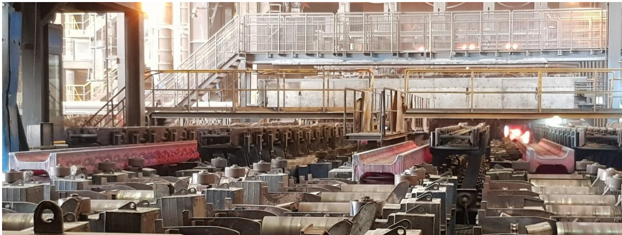
Fig: Meltshop Continuous Casting Machine (CCM)
